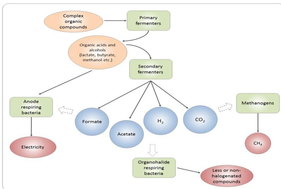
Fig. 3: Electron flow in anaerobic degradation of organic matter under different conditions
