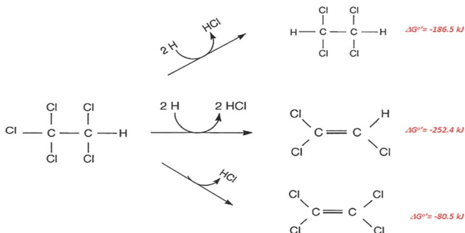
**Fig. 1: Examples of reductive dehalogenation of pentachloroethane to tetrachloroethane (Dofling, 2016)**
